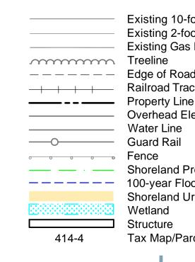
Existing 10-foot Contour Existing 2-foot Contour Existing Gas Pipe Edge of Road Railroad Track **Overhead Electrical Lines** Water Line Guard Rail Shoreland Protection Buffer 100-year Floodplain Shoreland Urban Exempt Area Structure Tax Map/Parcel No. Designation
